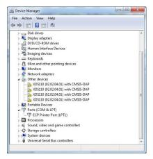
The Debug DevPack is using the XDS110 debug probe. This debugger is supported by a number of tools.
