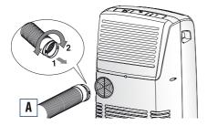
Screw the window outlet 17 to the other end of the exhaust hose. (see fig. B).
