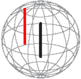
An Isotropic Antenna is a theoretical antenna that radiates a signal equally in all directions.
