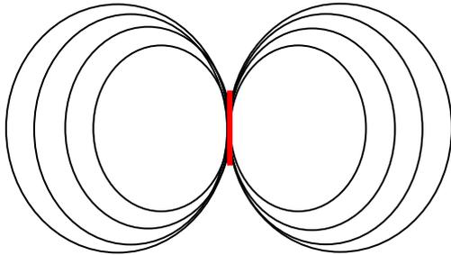
A Dipole Antenna is commonly used in wireless systems and can be modeled similarly to a doughnut
