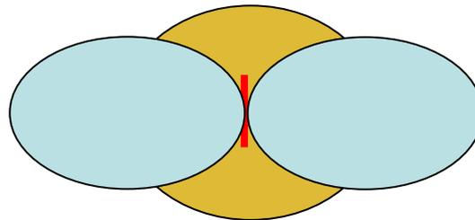
The Dipole represents a directional antenna with a further reach in the X&Y Plane (at the cost of a smaller reach in the Z plane) to the Isotropic.
