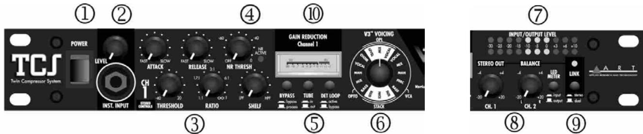
① **Power** – Switches the unit’s power on and off.
