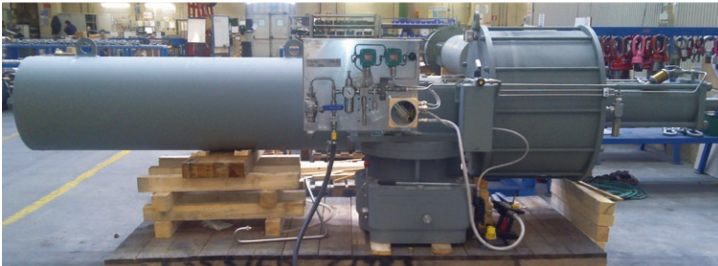
DYNATORQUE D-Stop partial-stroke test device direct-mounted to a LEDEEN pneumatic actuator
