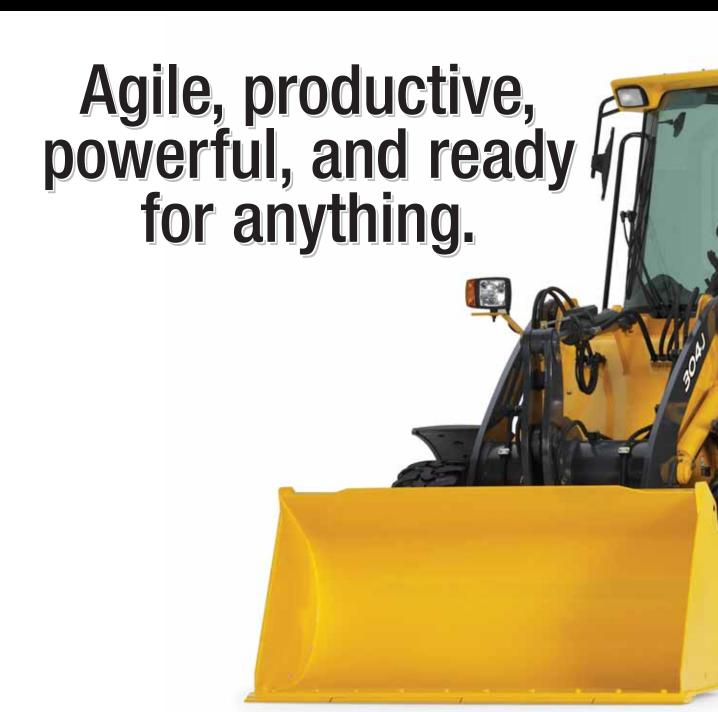
Need a compact loader to get big results? Choose the 304J. This versatile 73-hp machine combines outstanding maneuverability, travel speed, breakout force, reach, and stability in an innovative package. Its oscillating stereo steering delivers a turning radius that's 20-percent tighter than comparable loaders for fast work cycles.
