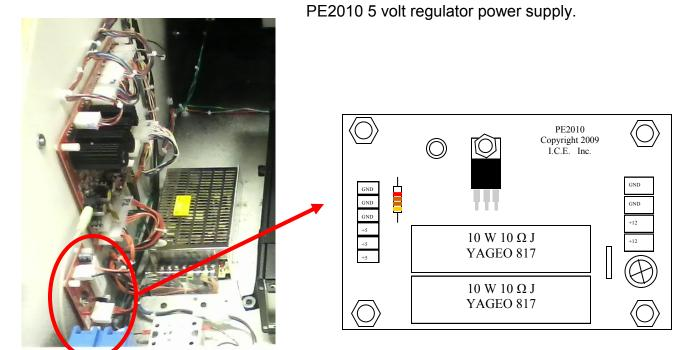
+5 volt regulator PCB. Incoming voltage is +12 volts of DC. Output is +5 DC regulated. If there is no +5 out check for +12 DC in or +12 out from PE2010X. If +12 is also missing, check 110v in to PE2010X power supply.
