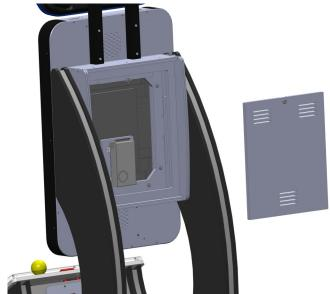
Remove the 14 screws holding the monitor to the cabinet. With a second person, push slightly from the back while someone from the front catches the monitor at the bottom as it slides out.
