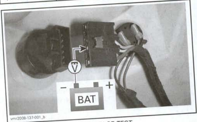
IGNITION SWITCH INPUT VOLTAGE TEST
