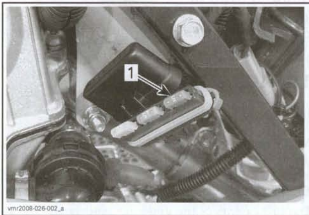
PF1 FUSE HOLDER 1. 5 A ECM fuse
