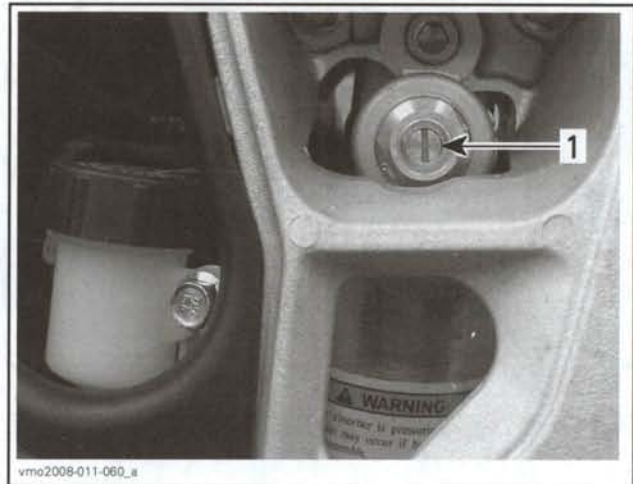
9 CLICKS COUNTERCLOCKWISE 1. Compression damping adjuster
