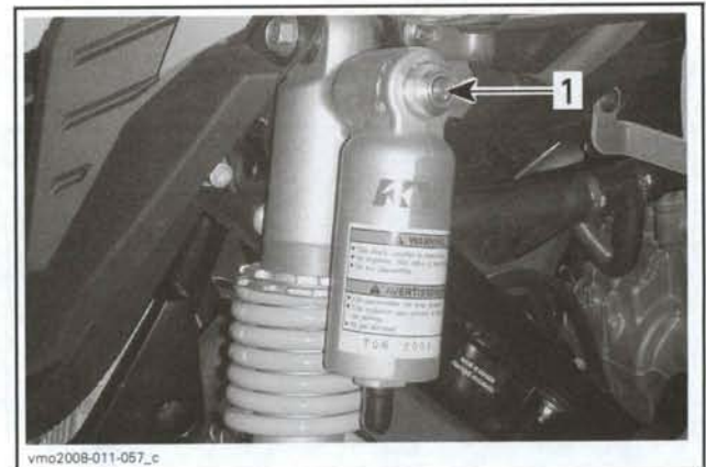
9 CLICKS COUNTERCLOCKWISE 1. Compression adjuster
