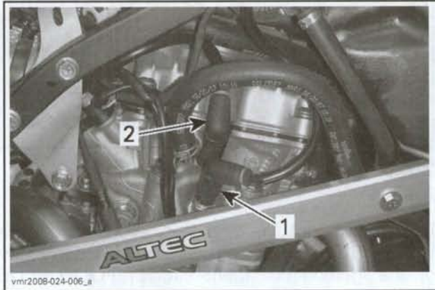
1. Outer spark plug cable to front coil 2. Inner spark plug cable to rear coil
