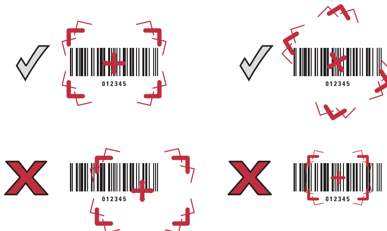
Figure 2-13 Acceptable and Incorrect Aiming
