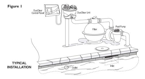
When the pump and filtration system is running, water that has passed through the pool filter is then passed through the DuoClear system.
