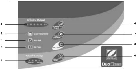
The "Chlorine Output" (6) controls the amount of chlorine generated by the electrode. Next to it are 6 indicator lights, (See power panel illustration above) I yellow (minimum output) and 5 green indicator lights (1). Maximum chlorine output is achieved when all lights are on.
