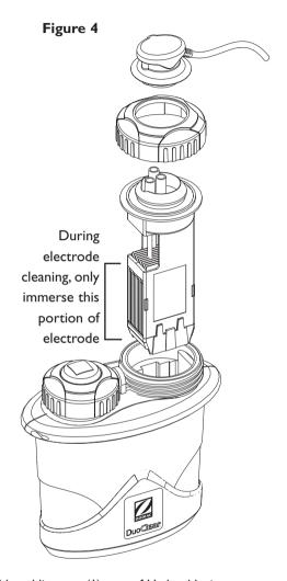
5. Mix cleaning solution in a suitable plastic vessel by adding one (1) part of Hydrochloric (muriatic) acid to ten (10) parts water. Note: To avoid splash, always ADD MURIATIC ACID TO WATER rather than water to muriatic acid. Solutions stronger than 1:10 will damage electrode and void warranty. Submerge only the plate of the electrode in the cleaning solution. See Figure 4. Allow the cleaning solution to dissolve the calcium deposits for approximately 5 minutes.
