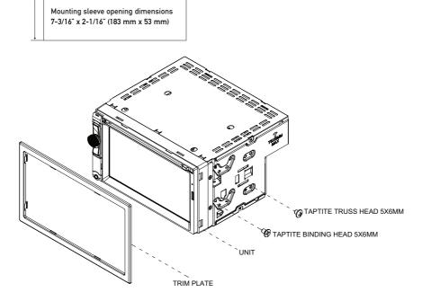
TYPICAL FRONT-LOAD DIN MOUNTING METHOD
