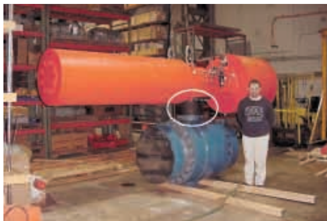
Figure 1: Typical example of a “sandwich-mount” product installed between the pneumatic actuator and valve.
