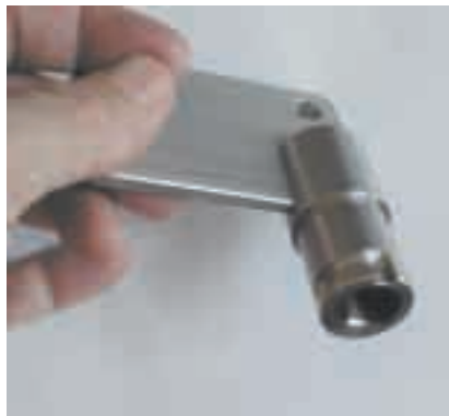
Figure 5: For manual operation, a controlled key is used to engage the Partial Stroke Test Device. The key cannot be removed from the mechanical testing device while it is in the test position. If plant operating personnel know the key is in their control and not in the test device, then they also know the device cannot be accidentally engaged.
