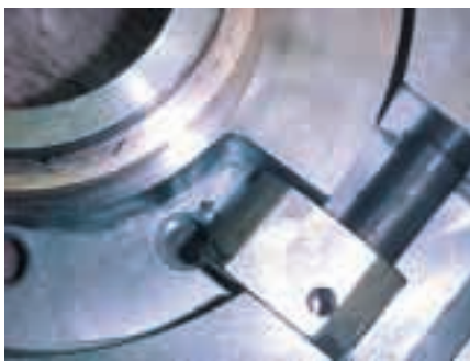
Figure 4: When a partial stroke test is required, the device is "engaged" and the ESD valve will only travel to the specified percentage of stroke. The device mechanically prevents movement past the interlock.
