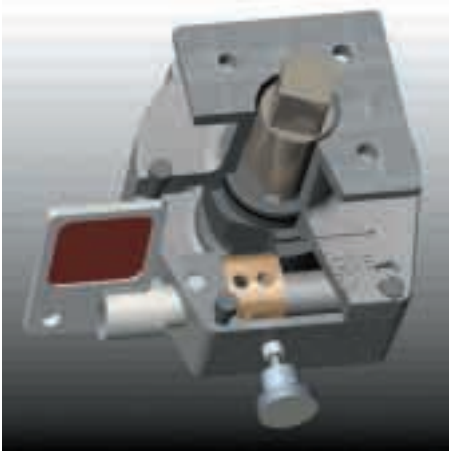
Figure 7b: ...the device is then “engaged” and maintenance informs the control room that the ESD is now ready to test.
