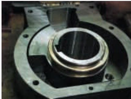
Figure 2: Fabricated body of a Partial Stroke Test Device. Valve Stem would be connected to the device through the bore and keyway.
