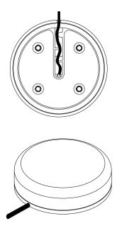
After drilling the holes, pass the o-ring over the antenna cable and press it into the groove on the bottom of the antenna housing. Now attach the antenna to the mounting surface, using 4mm screws and the supplied lock washers. Route the cable to the Eagle View and the antenna installation is finished.
