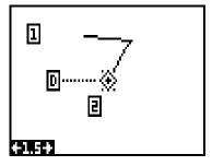
you recalled the waypoint. The dotted line is called a track line and is the shortest path from the starting location to the destination. The "D" is the cursor destination, the number with a box around it is the waypoint. If you follow the track line, you'll reach the destination, covering the shortest distance in the least time.
