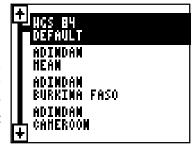
The WGS-84 label is highlighted. To change it, simply press the up or down arrow keys to highlight the desired datum, then press the ENT key. This selects the datum and erases the select datum menu.
