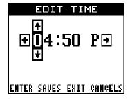
the up or down arrow keys until the desired number shows. Continue until the time shown in the display is correct, then press the ENT key. This enters the new time and clears the set clock menu.
