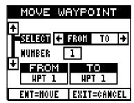
shown at right. Press the down arrow key, then press the right arrow key until the desired waypoint number shows in the box. When everything on this page is correct, press the ENT key.
