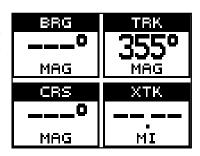
ror (XTK) are all shown on this screen. You must recall a waypoint to use the bearing, course, and cross track error windows. As you wait for the Eagle View to find your position, you'll see numbers flashing on the display. Anytime you see flashing numbers, it means the Eagle View does not have a position! Do not rely on any data that is flashing! When the numbers stop flashing, the unit has locked on to the satellites and the position is good.
