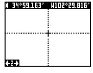
it's turned on, the zoom-in and zoom-out keys work from the cursor's position - not the present position, so you can zoom in on any detail, anywhere while navigating. The latitude/longitude of the cursor shows in the box at the top of the plot-1 screen whenever the cursor is activated. The cursor is also used to place and erase icons and waypoints.
