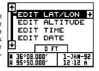
To change the position, press the right arrow key while the "EDIT LAT/LON" box is highlighted. The screen shown at right appears.
