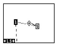
and a dashed line from the first waypoint to each of the other waypoints in the route. When you enter the radius set by the arrival alarm, the Eagle View automatically switches to the next waypoint on the list, showing navigation data to that waypoint, and so on until the last waypoint on the route list has been reached. (Note: The arrival alarm does not have to be turned on in order to use the route feature.)
