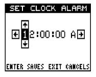
arrow keys until the desired number shows. Continue until the time shown in the display is correct, then press the ENT key. The alarm is now set.
