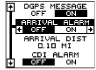
To use any of these alarms, first press the MENU key, then select the "ALARMS/CDI" menu. A screen similar to the one shown at right appears. Press the up or down arrow key to move the black box to the desired alarm, then press the right arrow key to turn it on.
