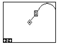
Every time you save a waypoint, the date and time are logged along with the position data. It's also placed on the plotter as shown above. In this case, waypoint number one was assigned when we quick-saved our position.
