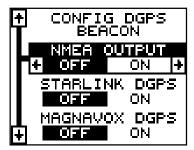
ment works, then no setup will need to be performed. If your other equipment doesn't recognize the NMEA data being sent by the Eagle View and the wiring is correct, then you may need to change the NMEA or the serial communication settings.
