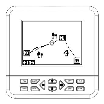
The WPT key lets you create, save, and recall waypoints and routes. The MODE key switches the unit between the three major displays: windows, navigation, and plotter. To select different features, or to modify functions, press the MENU key. The Z-IN and Z-OUT keys zoom-in and zoom-out your view on the plotter screen. The ENT and EXIT keys let you enter or erase selections. The PWR key turns the Eagle View on and off.
