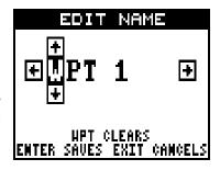
Press the up or down arrow keys to select the first letter in the name. Press the right arrow key to move the black box to the next position in the name. Repeat this sequence until you've entered all of the letters in the waypoint name. Press the ENT key to accept this name, the WPT key to erase all characters in the name, or the EXIT key to leave this screen without saving any changes.
