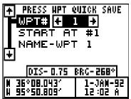
You can select any waypoint as the simulator's starting point. Select the starting point by pressing the right arrow key on the "WPT#" label until the desired starting waypoint number appears. Now highlight the "Start At" label and press the right arrow key. The Eagle View returns to the Simulator Setup menu.
