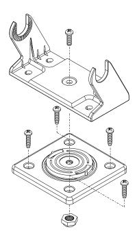
Attach the Eagle View to the gimbal bracket using the supplied gimbal knobs and washers as shown below.
