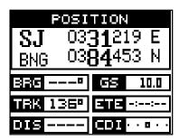
The Eagle View can use the military grid reference system (MGRS). It uses two grid lettering schemes, which are referred to as standard and alternate MGRS on the View. Your position and datum in use determines which one to use. In general, if the datum you're using is valid for your present position, then use the standard MGRS, otherwise use the alternate MGRS.
