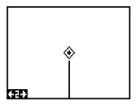
plotter's range is shown in the lower left corner of the screen. In this example, the plotter's range is two miles from the left edge of the screen to the right.
