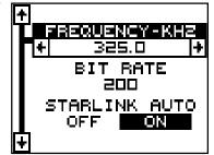
These menus select the beacon receiver's frequency and bit rate (in bits per second). If you are using a Starlink receiver, turning the auto mode on causes the Eagle View to auto-detect the frequency and bit rate.
