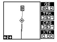
row key to move the black box to the "PLOT" label. Now press the right arrow or left arrow key to select plot 2. This screen (as shown at the bottom of the previous page) has navigation data displayed on the right side of the screen in digital numbers. This data is active whenever you've recalled a waypoint. Press the EXIT key to erase the mode menu.
