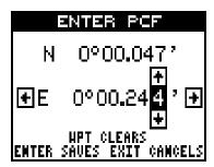
After you've entered the latitude/longitude correction, press the ENT key to accept it. The Eagle View erases the PCF entry screen and returns to the navigation or mapping screens with the correction factor applied.
