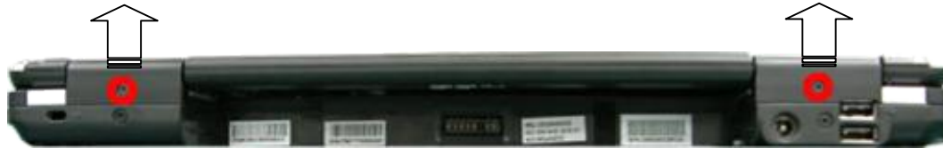
Fig. 25 Releasing LCD hinge cover
