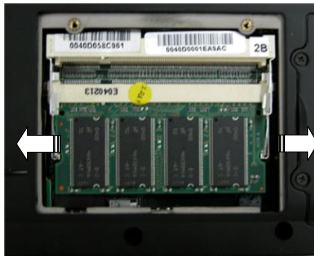
Fig. 10 Removing the memory module
