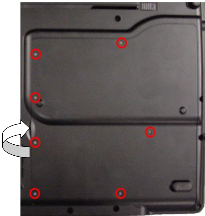
Fig. 8 Removing the screws retaining the memory module slot cover
