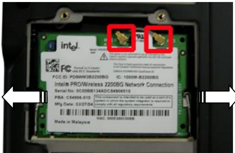
Fig. 12 Removing the WLAN module
