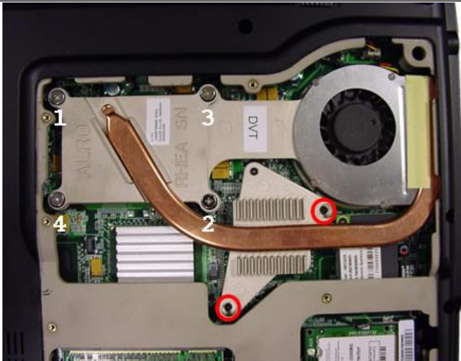
Fig. 16 Removing the heat sink
