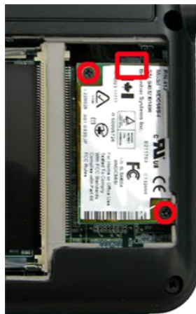
Fig. 13 Removing the MDC Modem module
