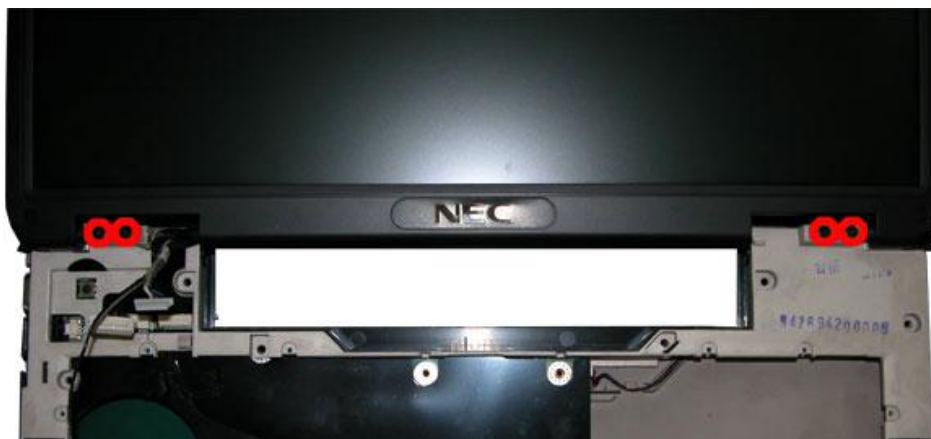
Fig. 28 Releasing the LCD Hinges
