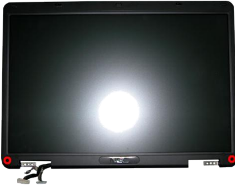
Fig. 29 Screws on the LCD Module
