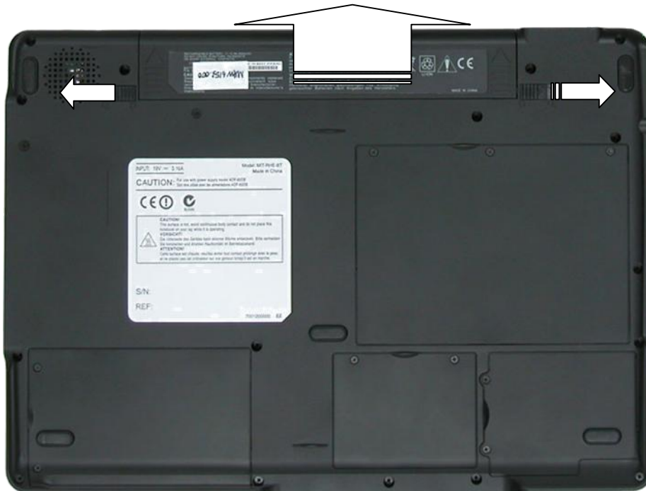
Fig. 1 Removing the battery
