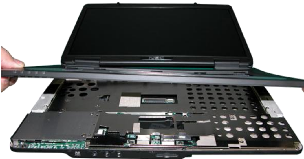
Fig. 24 Removing the Top Cover
