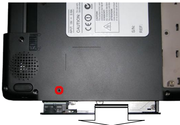
Fig. 6 Removing the optical drive
