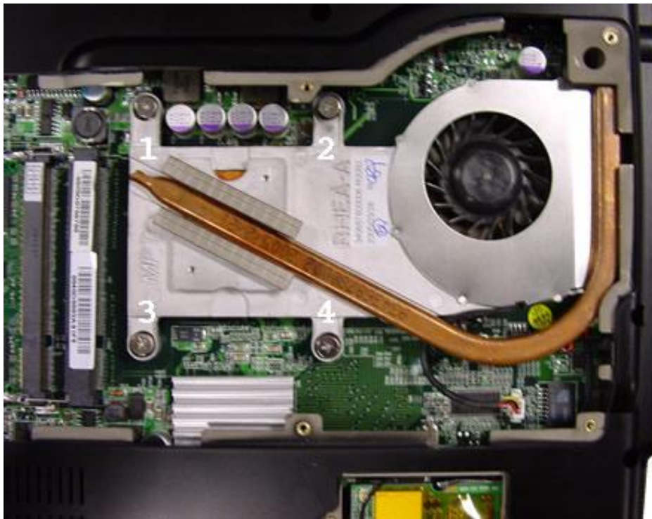
Fig. 17 Removing the heat sink
