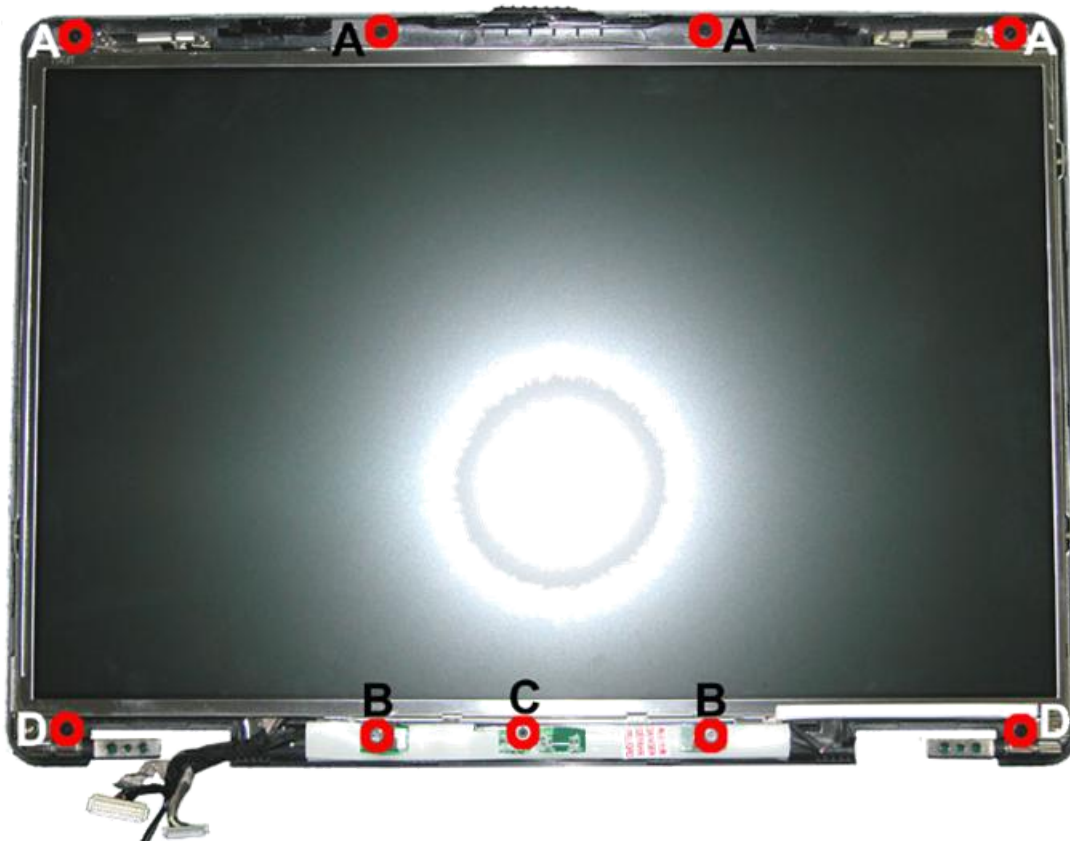
Fig. 31 Removing the LCD panel screws
