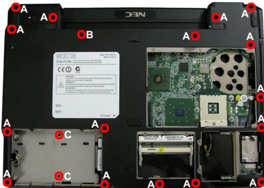
Fig. 22 Removing the top cover screws
