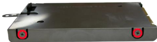
Fig. 5 Unscrewing the hard disk drive shield screws
