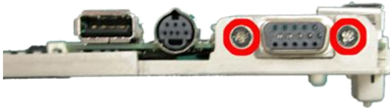
Fig. 37 Releasing System Bracket
