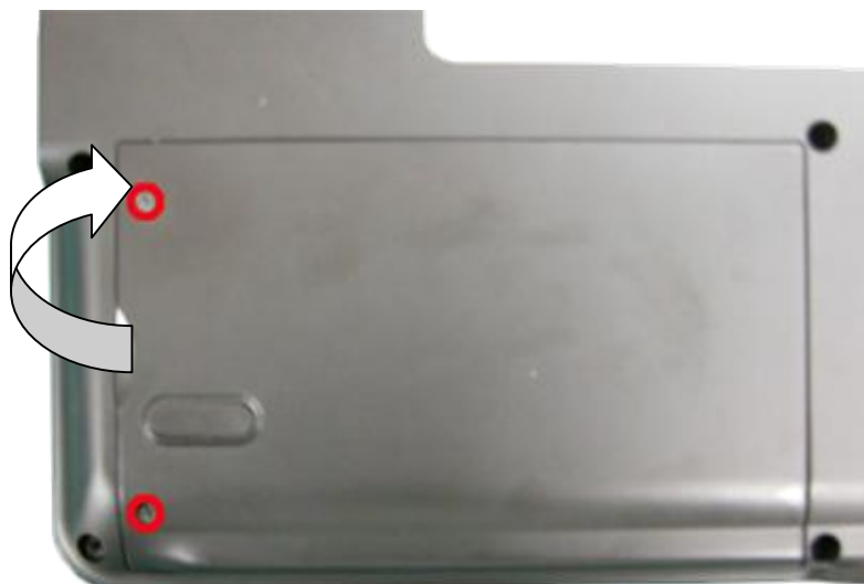
Fig. 3 Removing the Hard disk drive cover
