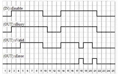
Figure 8: "WagoEnable" State Diagram
