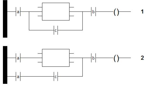
Figure 12: Ladder Diagram - Branch Variants
