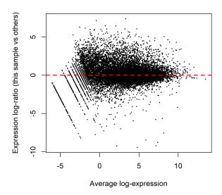
Ideally, the bulk of genes should be centred at a log-fold change of zero. This indicates that any composition bias between libraries has been successfully removed. This quality check should be repeated by constructing a MD plot for each sample.
