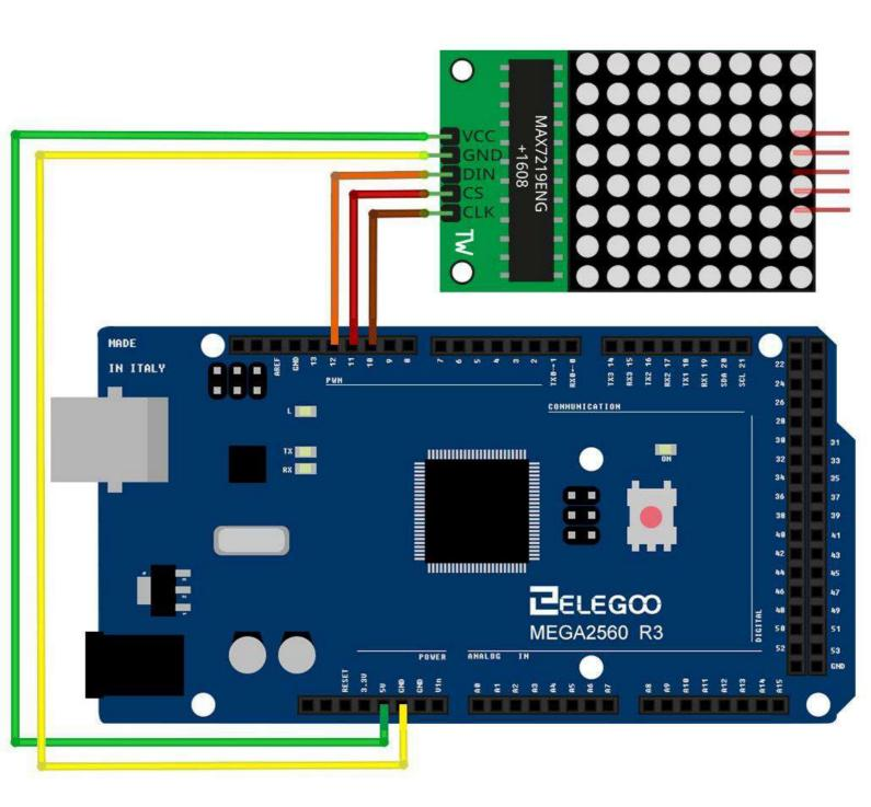
VCC and Ground are connected to the Arduino.
