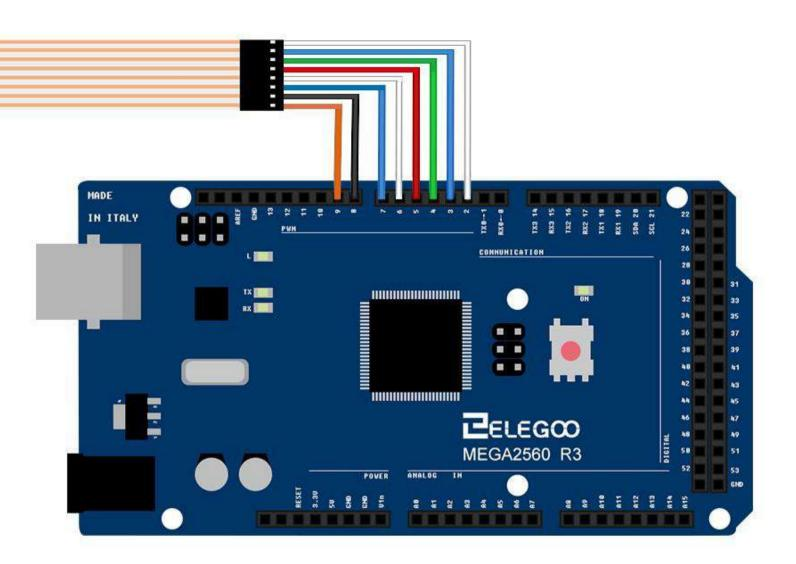
When connecting the pins to the MEGA2560 R3 board, we connect them to the digital output pins, D9-D2. We connect the first pin of the keypad to D9, the second pin to D8, the third pin to D7, the fourth pin to D6, the fifth pin to D5, the sixth pin to D4, the seventh pin to D3, and the eighth pin to D2.
