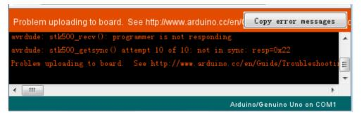
It can mean that your board is not connected at all, or the drivers have not been installed (if necessary) or that the wrong serial port is selected.
