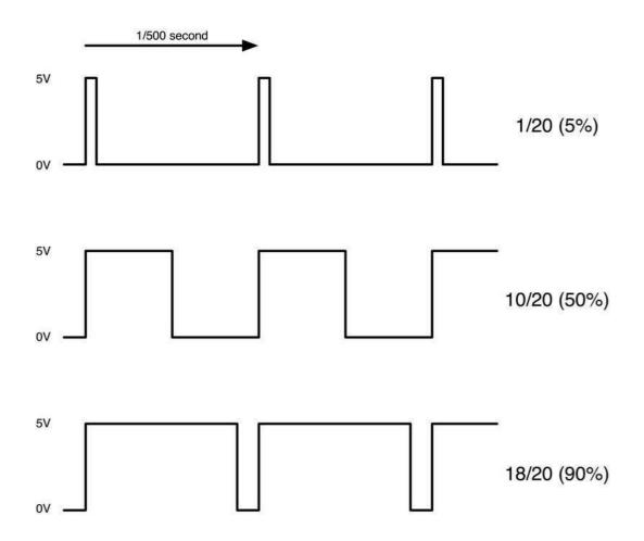
Roughly every 1/500 of a second, the PWM output will produce a pulse. The length of this pulse is controlled by the 'analogWrite' function. So 'analogWrite(0)' will not produce any pulse at all and 'analogWrite(255)' will produce a pulse that lasts all the way until the next pulse is due, so that the output is actually on all the time.
