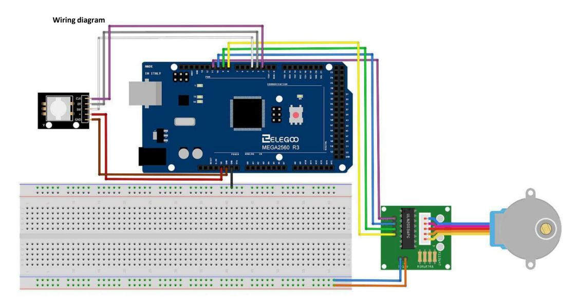
We are using 4 pins to control the Stepper and 3 pins for the rotary encoder module. Pins 8-11 are controlling the Stepper motor and pins 2-4 are receiving information from the rotary encoder.
