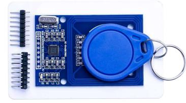
The MFRC522 is a highly integrated reader/writer for contactless communication at 13.56 MHz. The MFRC522 reader supports ISO 14443A / MIFARE<sup>®</sup> mode.
