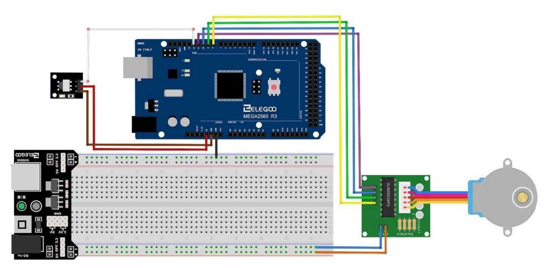
We are using 4 pins to control the Stepper and 1 pin for the IR sensor. Pins 8-11 are controlling the Stepper motor and pin 12 is receiving the IR information.
