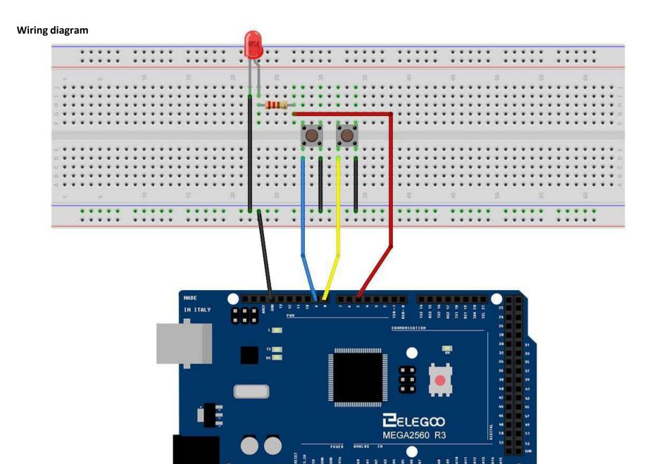
Although the bodies of the switches are square, the pins protrude from opposite sides of the switch. This means that the pins will only be far enough apart when they are placed correctly on the breadboard.
