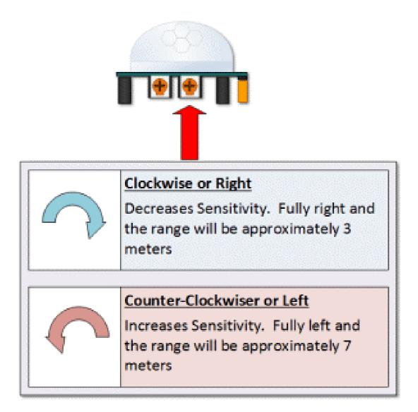
HC SR501 Sensitivity Adjust Time Delay Adjustment
