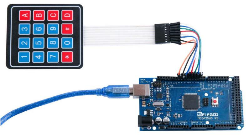
With this code, once we press a key on the keypad, it should show up on the serial monitor of the Arduino software once the code is compiled and uploaded to the MEGA2560 R3 board.
