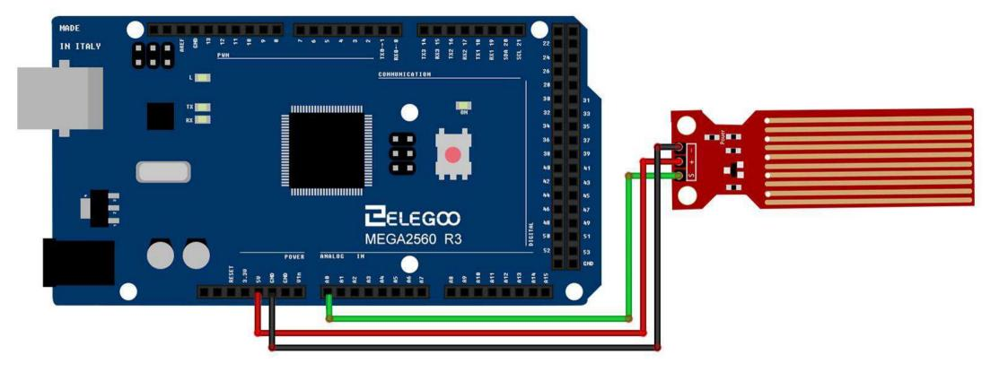
Wiring tips: Power supply (+) is connected to 5V of MEGA2560 R3 board, ground electrode (-) is connected to GND. Signal output (S) is connected to the ports (A0-A5) which have function of inputting analog signal in MEGA2560 R3 board, random one is OK, but it should define the same demo code as the routine.
