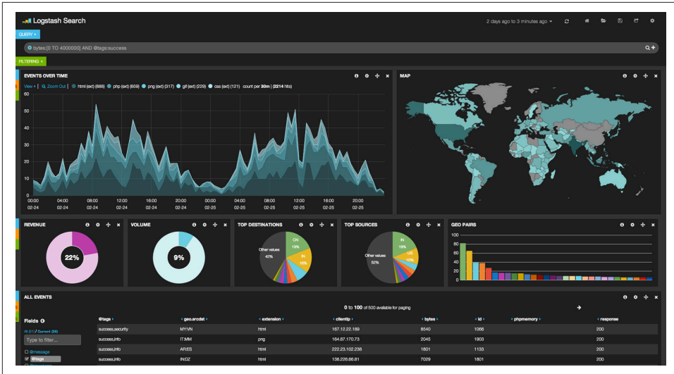
Figure 28-3. Kibana—a real time analytics dashboard built with aggregations
