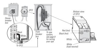
Carry out a visual inspection to check for signs of incorrect wiring.
