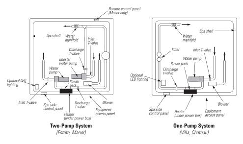
This diagram represents a generic one-pump and two-pump system. It is not intended to represent any specific model.
