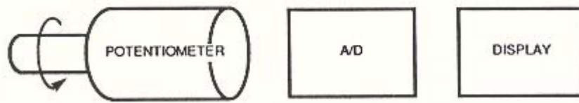
Figure 2-6. Measurement and Display of Rotary Displacement Using the Potentiometer
