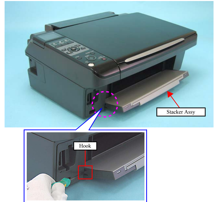
Figure 4-3. Removing the Stacker Assy
