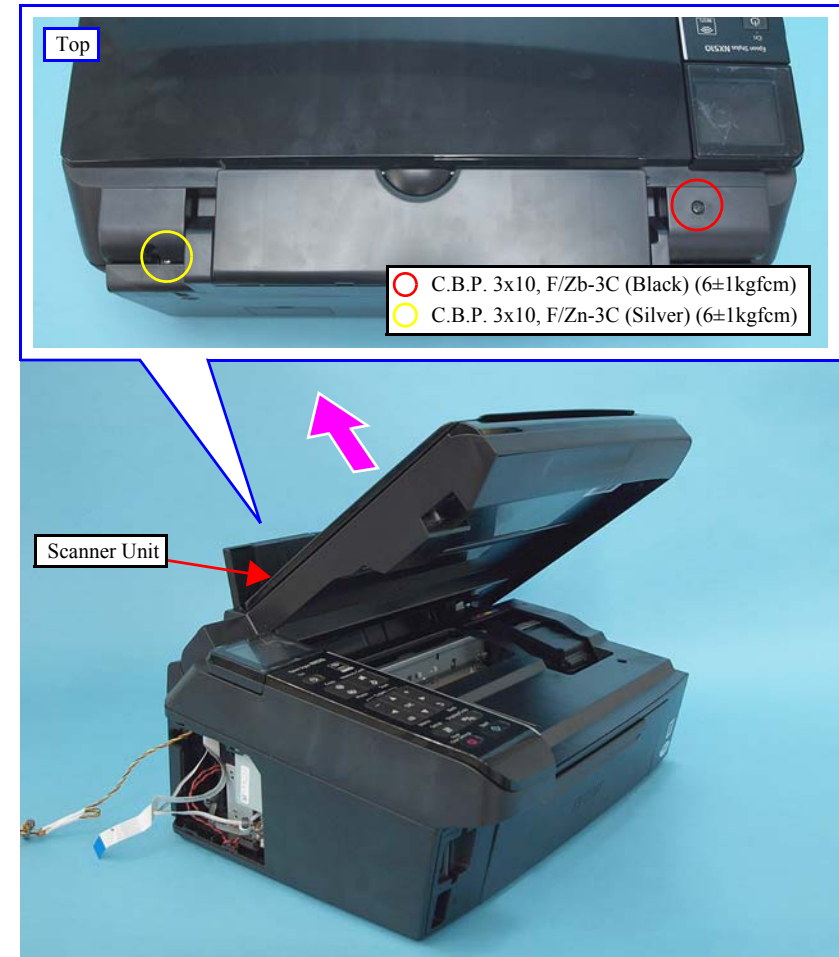
Figure 4-9. Removing the Scanner Unit (3)
