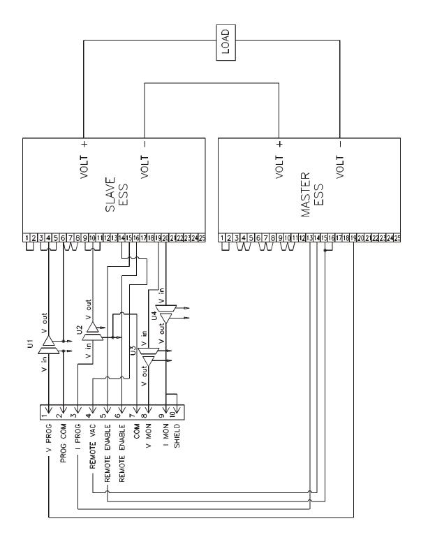
Figure 3.24 Series Operation with Opto Isolators
