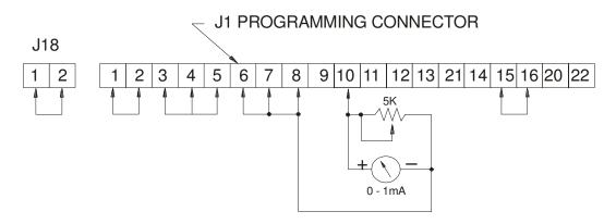
Figure 3.10: Remote Programming by External Current for Constant Current
