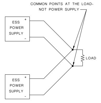
Figure 3.12: Parallel Operation
