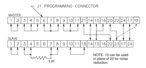
Figure 3.14.2: Paralled Operation in Master/Slave Configuration with OVP with Master On/Off Total Control Master/Slave and Higher Voltage Slave
