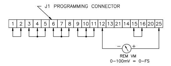
Figure 3.18: Remote Meter Across Shunt
