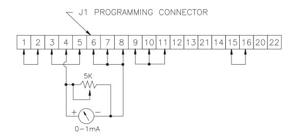
Figure 3.9: Remote Programming by External Current for Constant Voltage Current Channel
