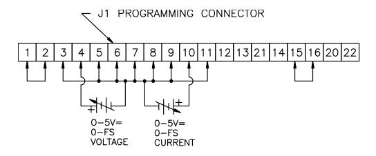
Figure 3.21: Remote Programming by External Voltage for Constant Current and Constant Voltage
