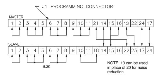
Figure 3.14.4: Paralled Operation in Master/Slave Configuration with OVP Total Control Master/Slave Local Control Note: Figure 3.78 and 3.8 for Voltage Current for Master on.
