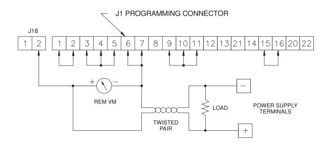
Figure 3.17: Remote Meter Across Load
