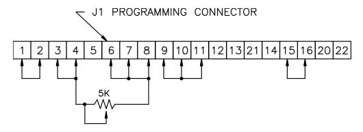
Figure 3.5: Remote Programming By External Resistance for Constant Voltage Current Channel
