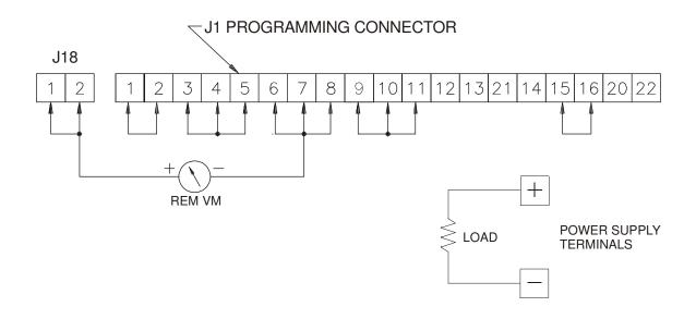
Figure 3.16: Remote Meter Across Output
