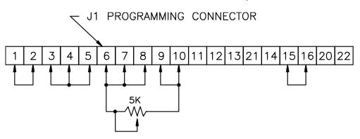
Figure 3.6: Remote Programming by External Resistance for Constant Current
