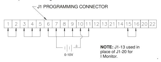
Figure 3.8: Remote Programming by External Voltage for Constant Current
