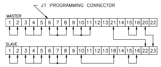
Figure 3.13: Parallel Operation in Master/Slave Configuration
