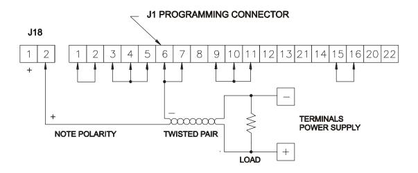
Figure 3.11: Remote Sensing
