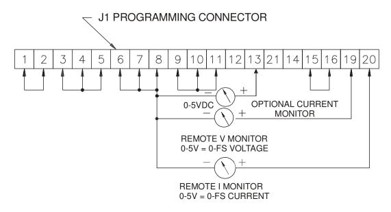
Figure 3.19: Voltage and Current Monitor
