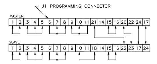
Figure 3.14: Paralleled Operation in Master/Slave Configuration with OVP Master/Slave
