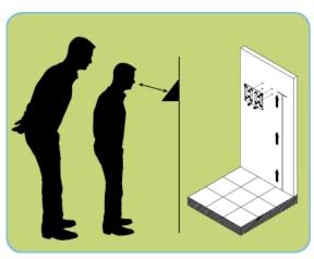
Install the mounting-plate to the wall using the supplied screws. For sheetrock walls, drill a 3/16" diameter hole through each of the four screw locations; each approx 1-1/2" deep. Install the plastic "anchors" included in the mounting screw packet.
