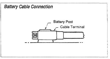
Poor contact at the battery cable connections is often a source of trouble. Make sure battery cables are in good condition and that contacting surfaces are clean and tightly connected. Do not reverse battery leads. Use recommended battery tools when disconnecting leads to avoid mechanical battery damage.
