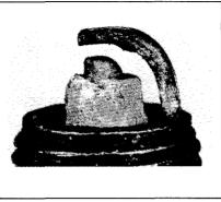
Worn: On a worn plug, the center electrode will be rounded and the gap will be eroded .010" or more than the correct gap. Replace a worn spark plug immediately
