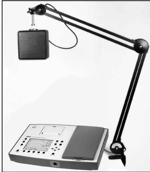
Figure 2.5.7—External sound field speaker setup
