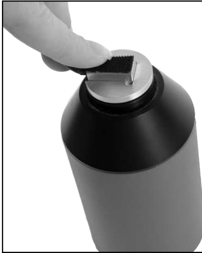
Figure C-5A: Rectangular reference microphone inserted into sound calibrator
