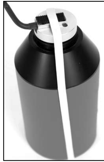
Figure C-5B: Using a rubber band to hold the microphone in place on the calibrator
