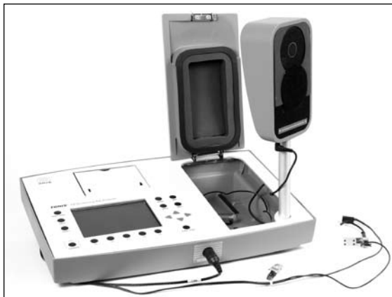
Figure 5.2.2—Internal sound field speaker setup
