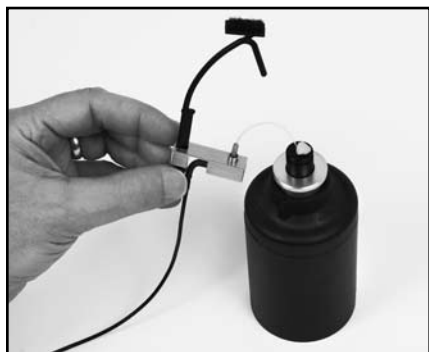
Figure C-4A: Integrated probe microphone inserted into sound calibrator.
