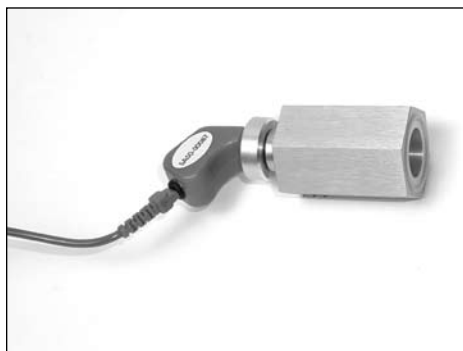
Figure C-8—Insert earphone connected to earphone calibration adapter and coupler
