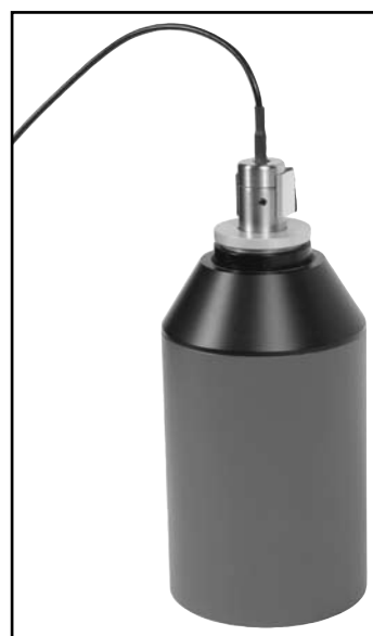
Figure C-3: Coupler microphone inserted into sound calibrator.
