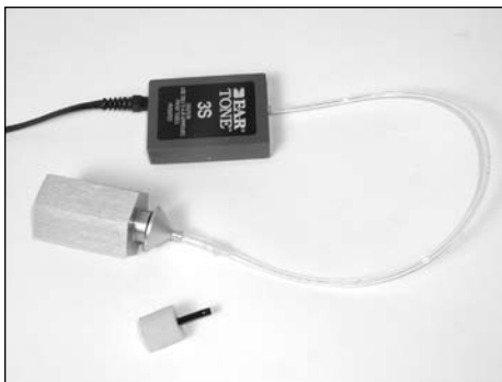
Figure C-6—Insert earphone connected to ear level adapter and HA-2 coupler
