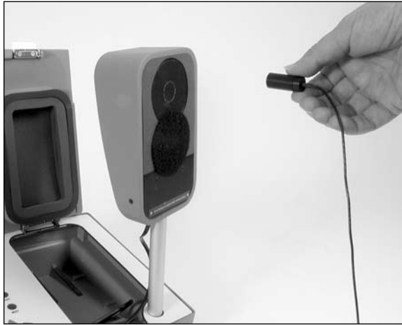
Figure 3.8.2B—Hold microphone six inches from the speaker
