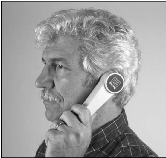
Figure 5.7.6A—Measuring telecoil response with the Telewand.
