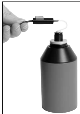
Figure C-4B: Old style probe microphone inserted into the sound calibrator.
