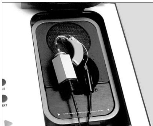
Figure 3.2.2—Leveling using the reference microphone
