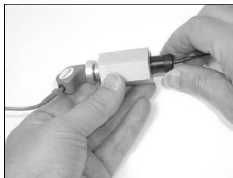
Figure C-9—Coupler microphone inserted into HA-2 coupler
