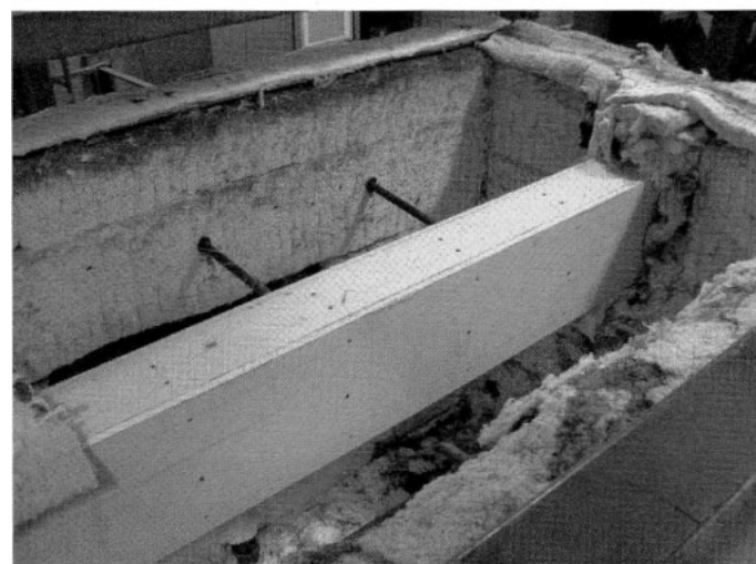
Figure 1. —Specimen in intermediate-scale horizontal furnace.
