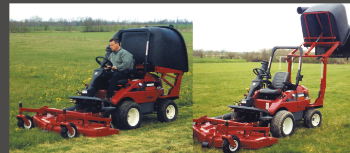
Flip-up mower deck Hydrostatic transmission Dual-element air filters
