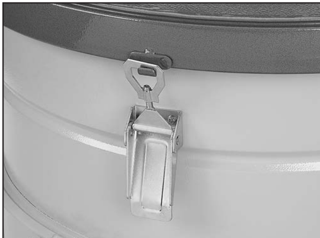
Figure 32. Latch hooked over the lid for clamping.
