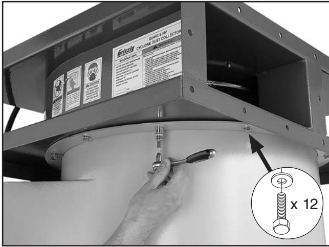
Figure 20. Securing blower on intake barrel.
