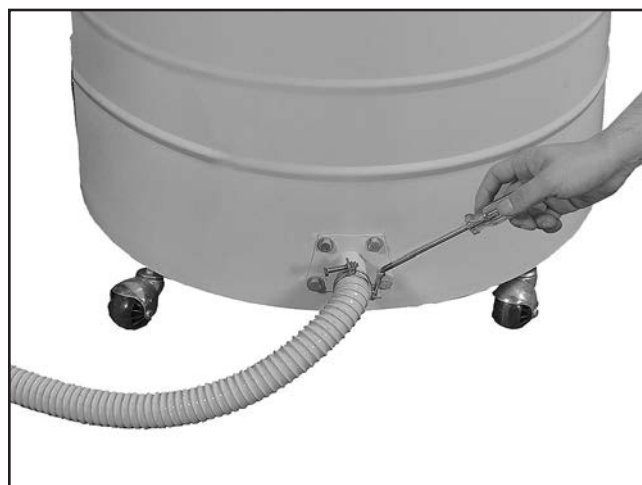
Figure 35. Connecting the vacuum hose.
