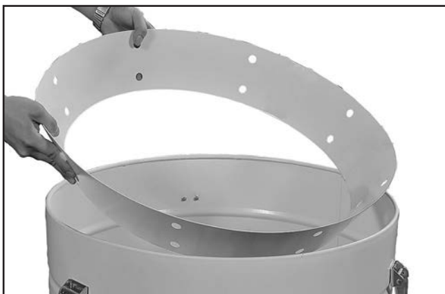
Figure 29. Inserting collection drum vacuum ring.
