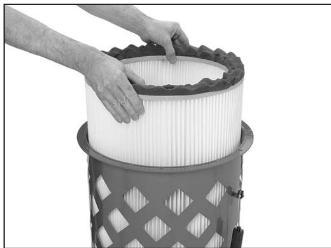
Figure 76. Removing the filter from the canister assembly.
