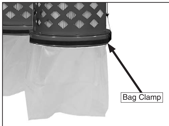
Figure 34. Canister filter collection bag installed.
