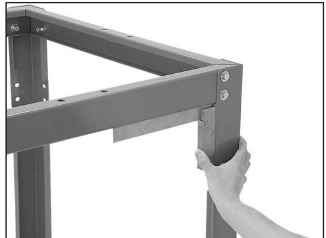
Figure 12. Squaring stand assembly before tightening stand hardware.
