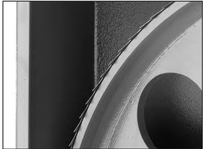
Figure 14. Blade positioned on wheel.
