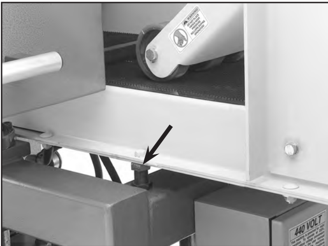
Figure 39. Conveyor table adjustment bolts (1 of 4 shown).
