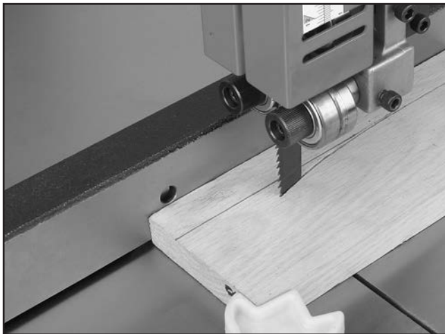
Figure 99. Blade leading away from line of cut.
