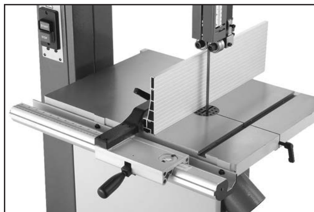
Figure 39. Correctly installed fence.
