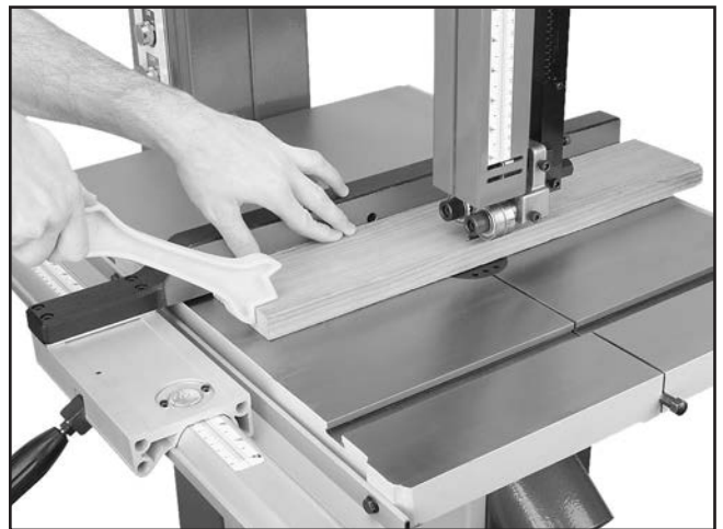
Figure 74. Ripping with a push stick.
