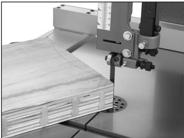
Figure 77. Typical stacked cut.
