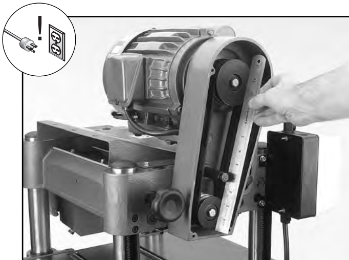
Figure 19. Checking pulley alignment.
