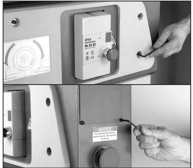
Figure 17. Removing cover plates.
