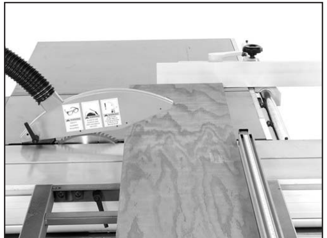
Figure 61. Correct rip fence position when using it as a cut-off gauge.
