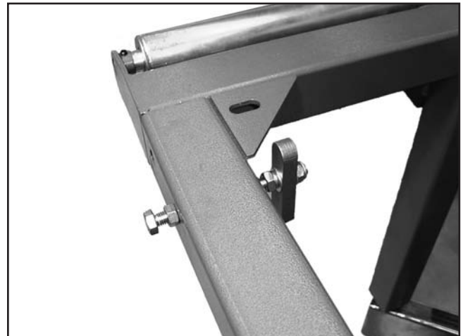
Figure 44. Crosscut fence adjustment screw.
