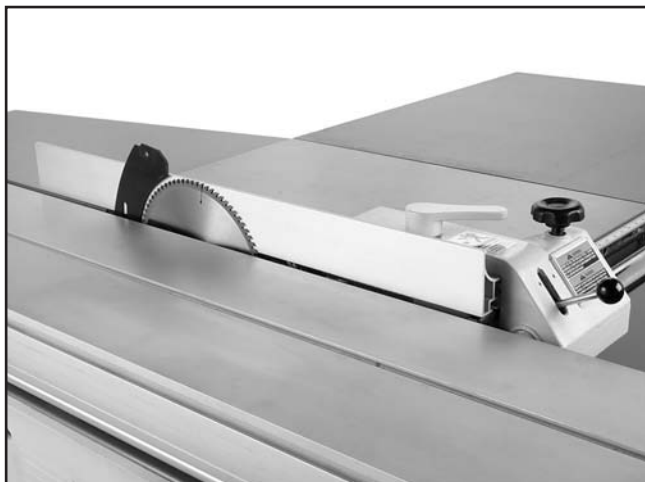
Figure 36. Fence against blade as a guide for aligning the scoring blade.
