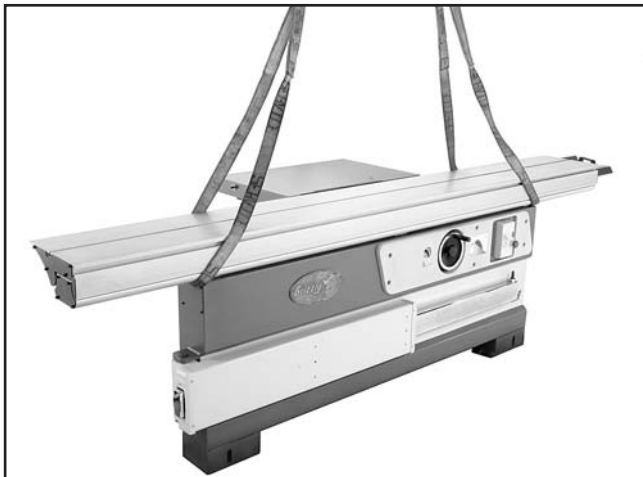
Figure 16. Installing the sliding table.
