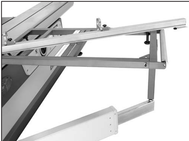
Figure 62. Fence set-up for 90° to 135° cuts.
