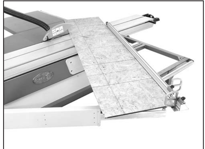
Figure 64. Example of miter cutting operation.
