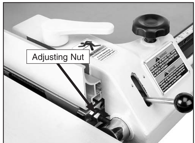
Figure 24. Aligning the round rail.
