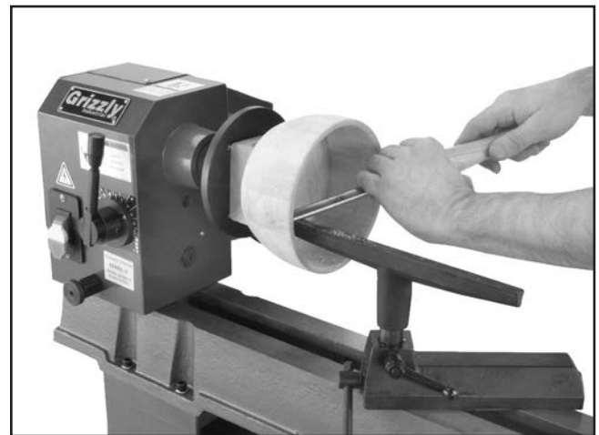
Figure 39. Typical faceplate turning operation.
