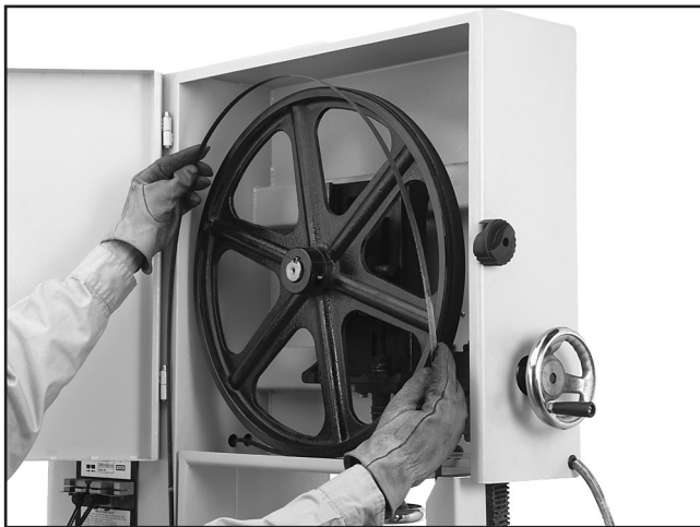
Figure 17. Placing blade on upper wheel.
