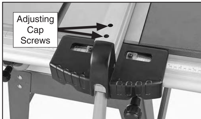
Figure 120. Location of cap screws for adjusting fence parallelism.
