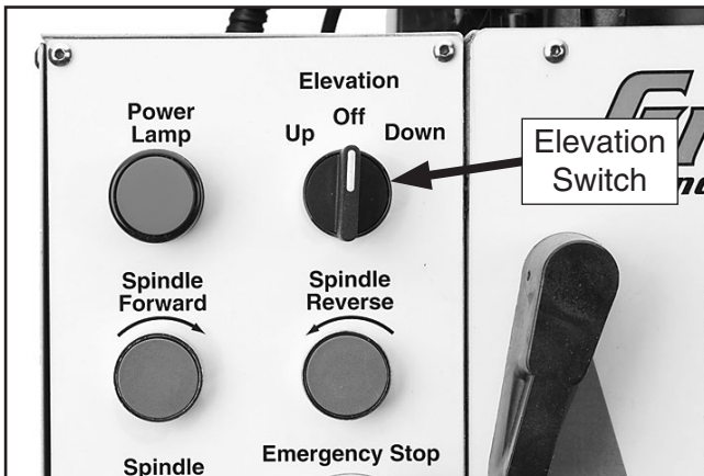
Figure 14. Elevation switch that controls motorized head travel.
