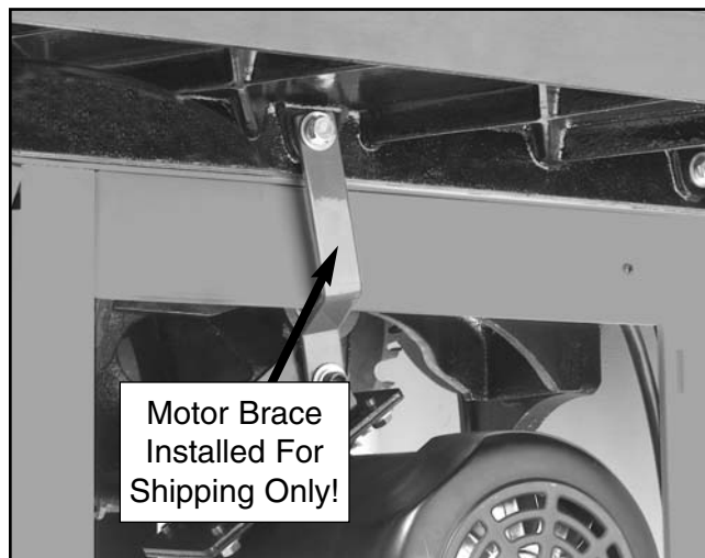
Figure 11b. Motor brace.
