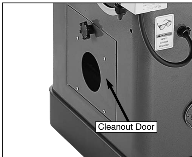
Figure 11a. Installed cleanout door.
