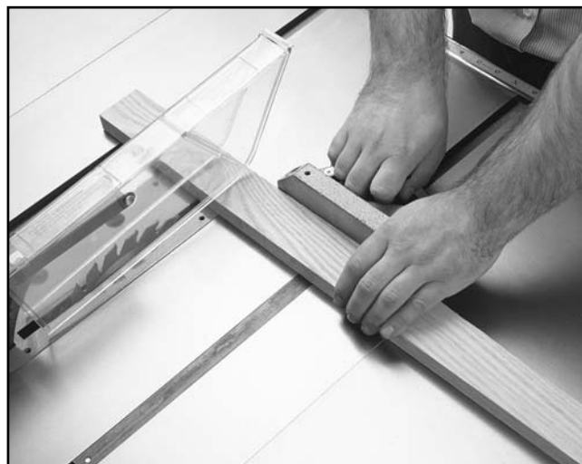
Figure 30. Typical cross-cut operation.
