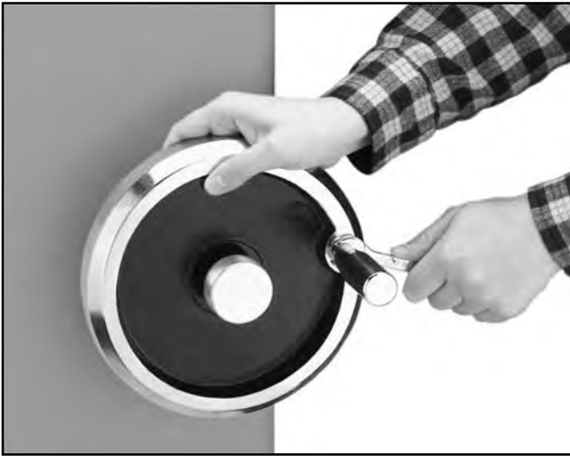
Figure 15. Tightening handle onto handwheel.
