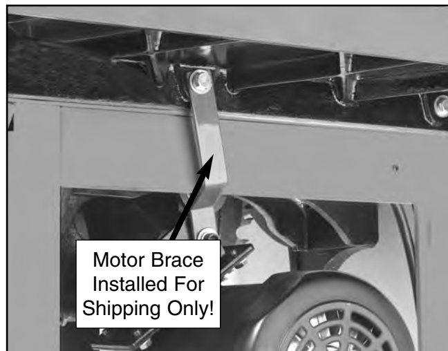
Figure 12b. Motor brace.
