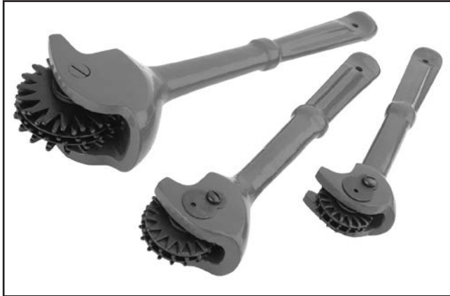
Figure 27. Rotary-type dressing tools.
