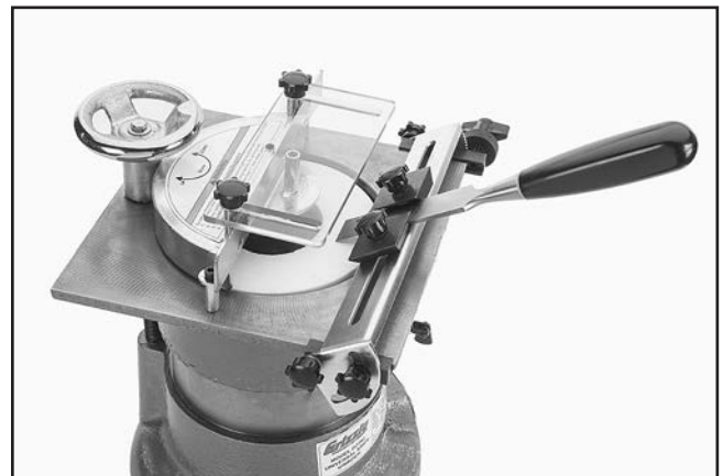
Figure 1. Example of a grinding setup for a chisel.
