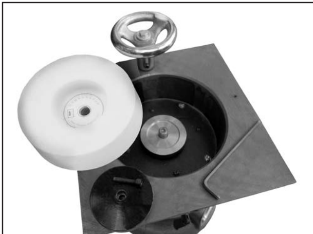
Figure 34. Grinding wheel removed from grinder.
