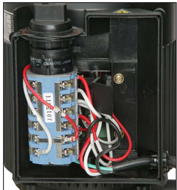
Figure 25. Motor switch (front view).
