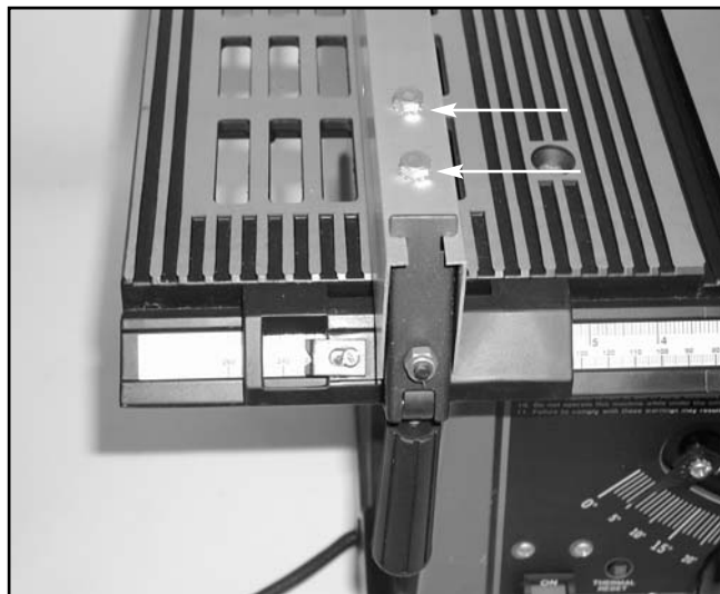
Figure 14. Fence adjustment bolts
