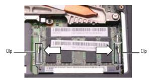
5 Pull the memory module out of the slot.
