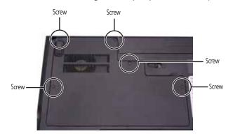
**3** Use the thumb notch to lift the cooling assembly bay cover, then remove it. Be careful not to break off the tabs located on the end of the cover opposite the thumb notch.
