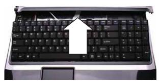
5 Slide the keyboard connector clip to the back of the notebook or lift the connector clip off of the cable, then slide the cable out of the clip. Be careful not to touch or damage any other components.
