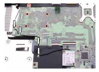
**16** Remove the screw holding the right speaker to the notebook, then remove the speaker.
