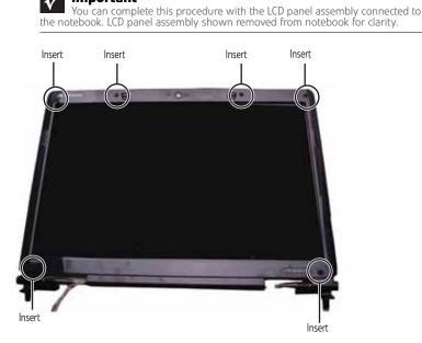
5 Remove the screws from the front of the LCD panel assembly.
