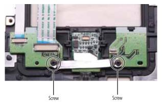
Swing the black fingerprint reader connector clip upward, then lift the cable out of the connector. Be careful not to touch or damage any other components.
