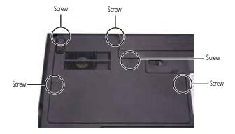
3 Use the thumb notch to lift the memory bay cover, then remove it. Be careful not to break off the tabs located on the end of the cover opposite the thumb notch.
