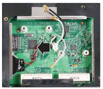
Lift the old battery off of the system board.
