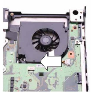
18 Remove the optional EMI shield screws.
