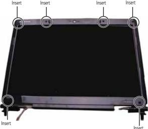
5 Remove the screws from the front of the LCD panel assembly.
