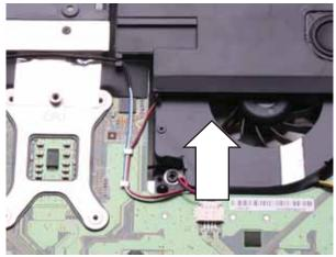
14 Remove the modem by following the instructions in "Replacing the modem" on page 121.
