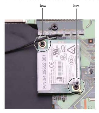
9 Lift the modem off of the system board.
