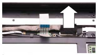
Taking care to note the cables' routing and positions as they are installed from Gateway, pull the antenna cables out from under the system board, then slide the antenna cables and LCD cables out from under the retaining clips. Remove any tape that may be securing the cables.
