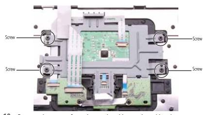
10 Remove the screws from the touchpad button board bracket.
