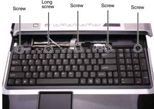
4 Lift the back edge of the keyboard slightly, then slowly slide it toward the LCD panel to release the keyboard retaining tabs located on the front edge of the keyboard.
