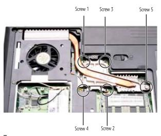
At the same time as you lift, move the main cooling assembly away from the side of the notebook, then remove the main cooling assembly.
