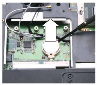
Make sure that the positive (+) side of the new battery is facing up, then press
