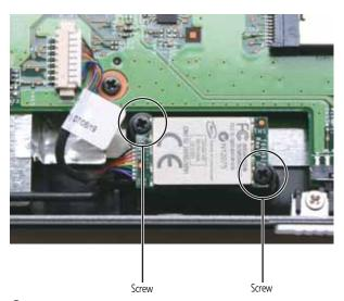
9 Disconnect the cable from the old Bluetooth module.
