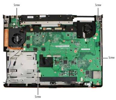
20 Carefully remove the system board.
