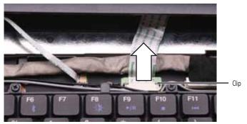
**Optional:** Slide the white power button cable connector clip to the left of the notebook, then slide the cable out of the clip. Be careful not to touch or damage any other components.
