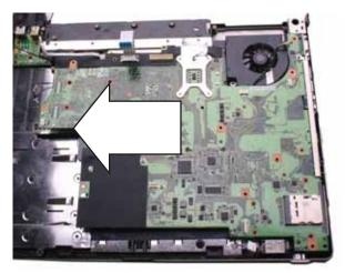
21 Turn the old system board over, then remove the optional second cooling assembly from the system board.
