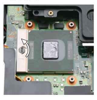
4 Remove the old processor from the system board.
