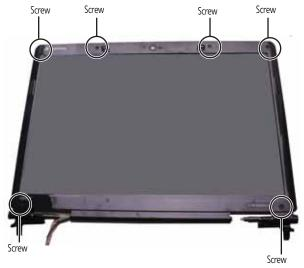
**6** Carefully separate the front and back of the LCD panel assembly.
