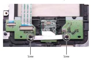
11 Swing the brown touchpad connector clip upward, then lift the cable out of the connector. Be careful not to touch or damage any other components.
