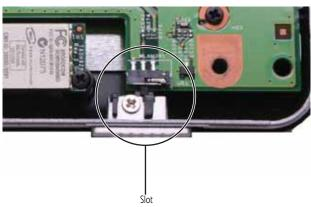
The connector between this board and the modem jack/USB board is fully connected.
