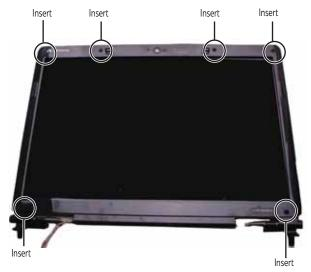
**7** Remove the screws from the front of the LCD panel assembly.
