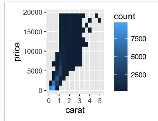
✓ To customize the plot, the following arguments can be used: *xmax*, *xmin*, *ymax*, *ymin*, *alpha*, *color*, *fill*, *linetype* and *size*.
