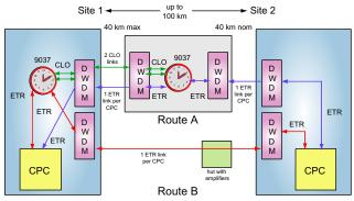
Note: Midspan 9037 can also be located within 40 km of site 2 or on Route B All ETR and CLO links are provisioned as 1 channel per wavelength.
