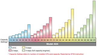
\* Capacity Setting refers to number of installed CPs and capacity. Reported by STSI instruction Note: For MSU values, refer to: ibm.com/servers/eserver/zseries/library/swpriceinfo/
