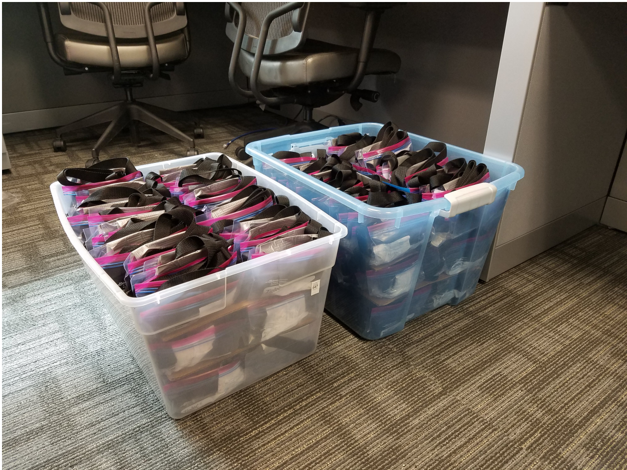
Figure 7: Two hundred AudioMoth housings made from Ziploc bags
