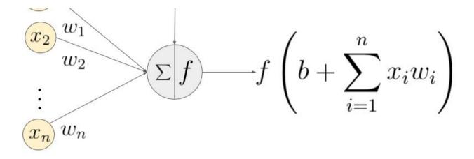
An example of a neuron showing the input ( $x_1 - x_n$ ), their corresponding weights ( $w_1 - w_n$ ), a bias (b) and the activation function f applied to the weighted sum of the inputs.
