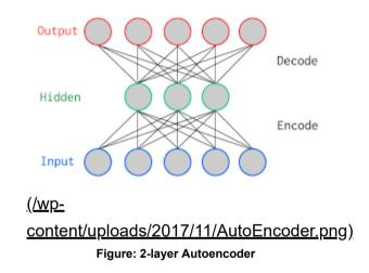
In the above picture, we show a vanilla autoencoder — a 2-layer autoencoder with one hidden layer. The input and output layers have the same number of neurons. We feed five real values into the autoencoder which is compressed by the encoder into three real values at the bottleneck (middle layer). Using these three real values, the decoder tries to reconstruct the five real values which we had fed as an input to the network.
