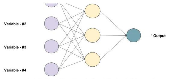
An example of a Feed-forward Neural Network with one hidden layer (with 3 neurons)
