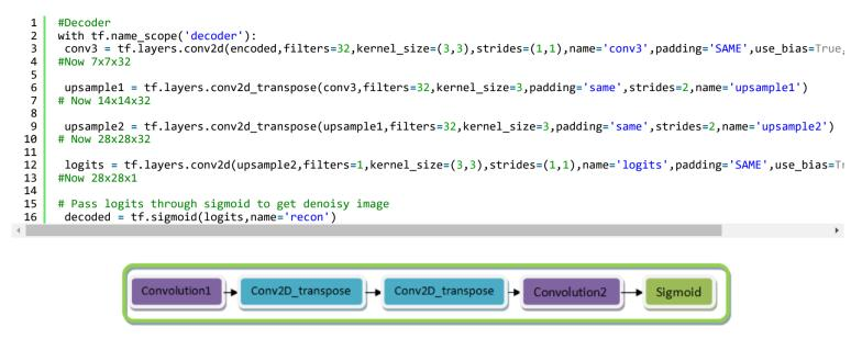
Figure: Decoder Block Diagram
