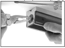
the included wrench. Move the bottom nut to adjust the level. Clockwise moves the nut down, and counter-clockwise moves it up. This level is so sensitive that resting your weight on the surface that you are leveling can affect the readings!
