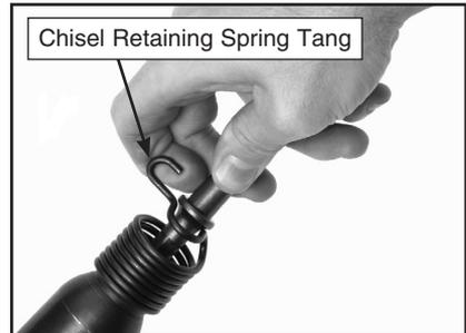
**Figure 3.** Chisel installation.
