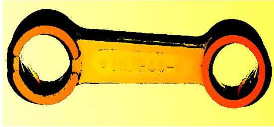
Figure 6.16: Result of uncalibrated sheet-of-light measurement: disparity image.
