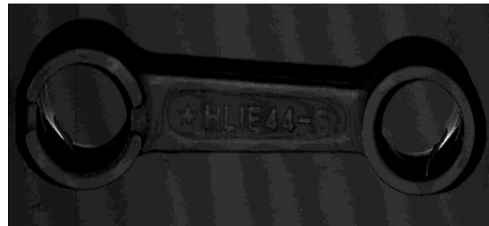
Figure 6.18: Result of uncalibrated sheet-of-light measurement: score image (score_type set to 'width', i.e., bright parts indicate artifacts).
