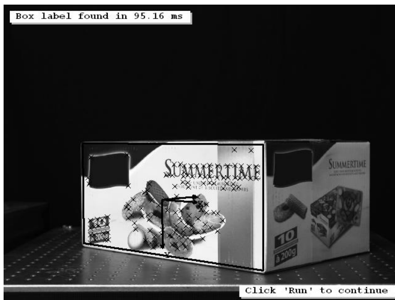
Figure 4.18: 3D pose of a cookie box label obtained by a calibrated descriptor-based matching.
